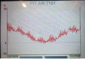
Graphs: Two online data loggers with temperature probes recorded ambient temperature (T103) and underground valve pit air temperature (T101). The graphs covered a year long of data starting from August 2014 to July 2015, data were collected once every hour.
